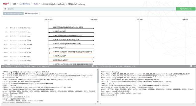
Signalling messages are displayed graphically in a sequence diagram. Permitting a clear presentation of the complete signalling traffic between the various components.
